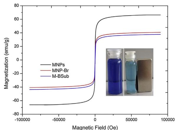
Fig. 3. Room-temperature magnetization curves for the MNPs, MNP-Br and M-BSub.
