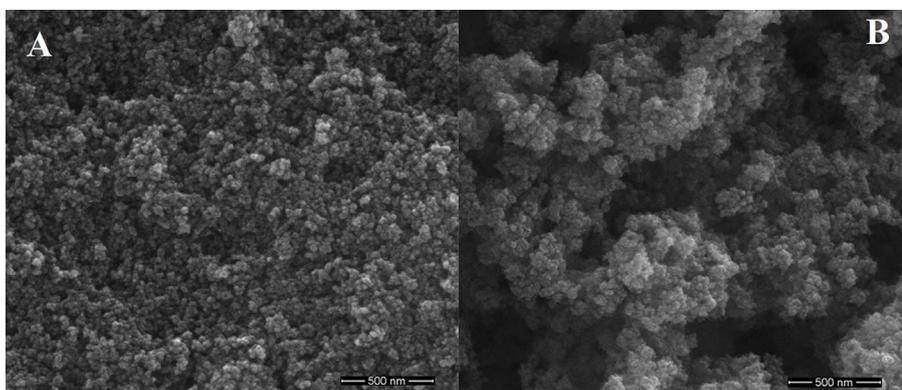
Fig. 4. A) SEM graphs of the M-BSub and B) MB biosorbed M-BSub.
