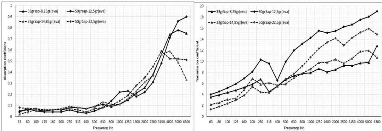
**Figure 4.** The effects of density and binding material to the sound absorption and sound transmission value in single-layer composite structure
