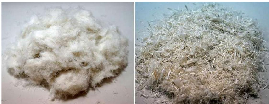
**Figure 1.** Fiber and rachis materials obtained from chicken feather fibers
