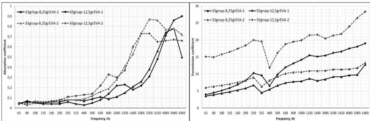
**Figure 5.** The effects of thickness and density to the sound absorption and sound transmission value in composite structures
