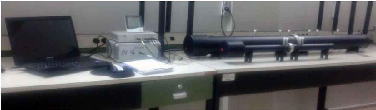
**Figure 3.** Impedance tube
