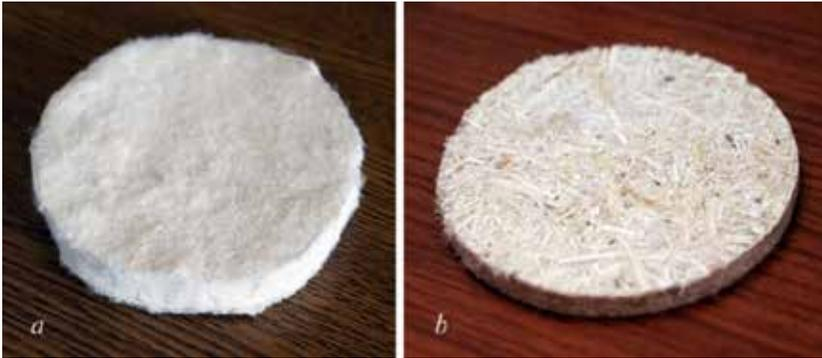
**Figure 2.** Samples produced out of CFF (a) and CFR (b)
