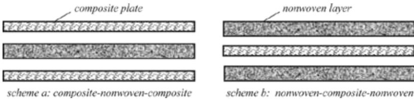
**Figure 5.** Schemes of preparing sandwich structures
