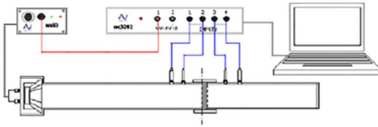
Figure 8. Sound transmission loss measurement
