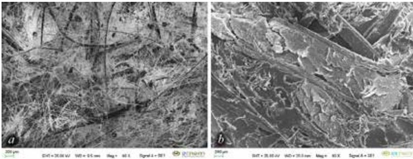
**Figure 3.** SEM image of the internal section of the nonwoven surface (a) and composite sample (b)
