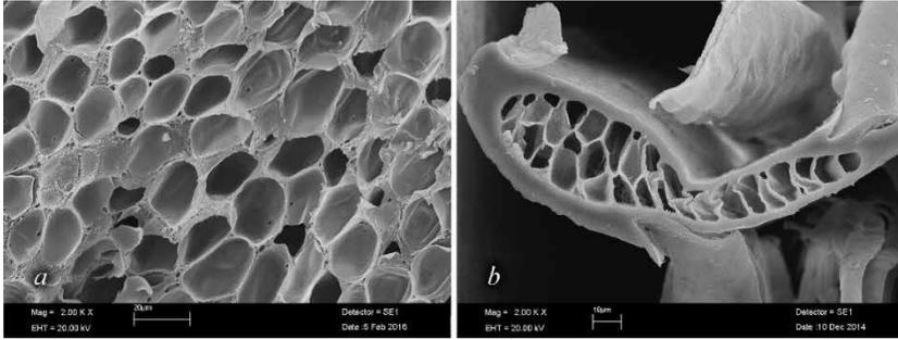
**Figure 1.** SEM images cross section of CFR (a) and CFF (b)
