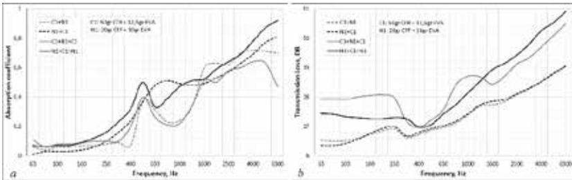
**Figure 10.** Acoustic curves of dual and triple combined structures with C1 and N1 content
