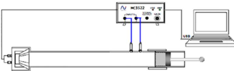
**Figure 7.** Sound absorption coefficient measurement
