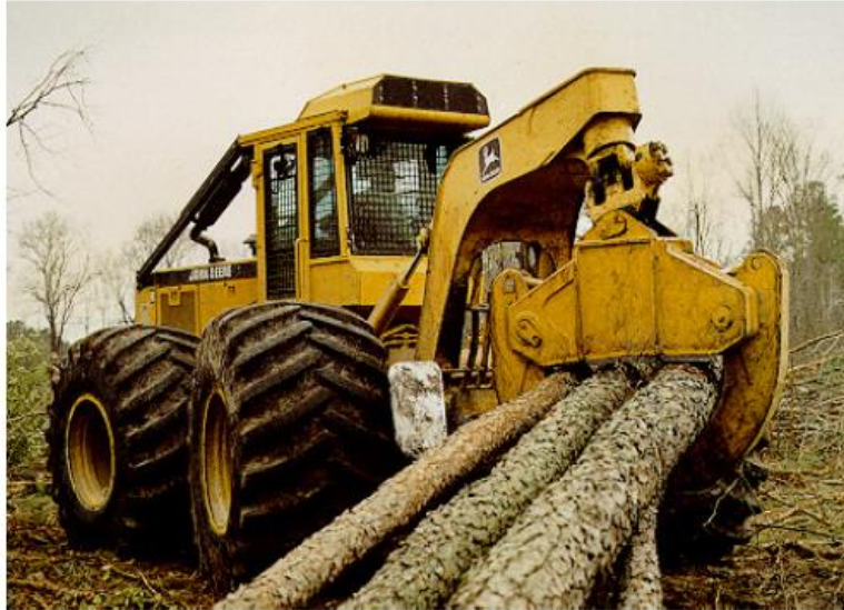
Figure1 — An example of a rubber-tired grapple skidder.
